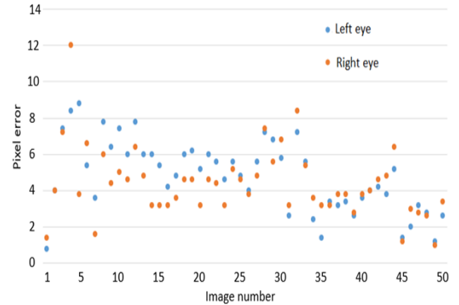
Figure 6. Left and right eye error for 50 images. (In this study, we evaluated images only from one camera to find the pupil location in 2D. However, one can easily employ off-the-shelf routines to find the location of the head position in 3D using images from two cameras.)
