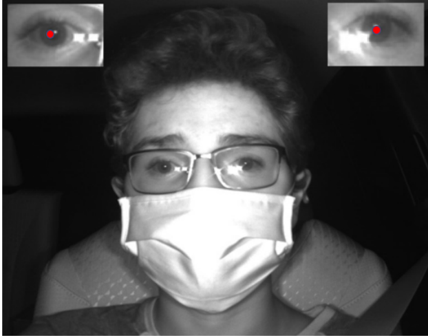
Figure 4. Nighttime driving. There are multiple reflections from the glasses in this example. Red dots show the detected pupil positions.
